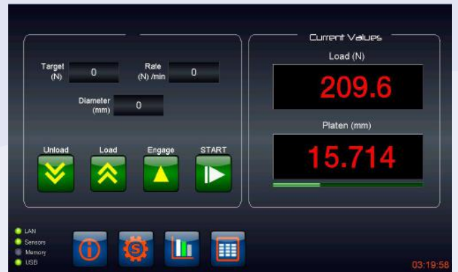
ACONS Pro "7" Touchscreen Colour Display Control Screen
