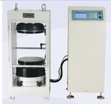
*VJT51-2011 - 2000kN Automatic Concrete Machine (Autocon)*
