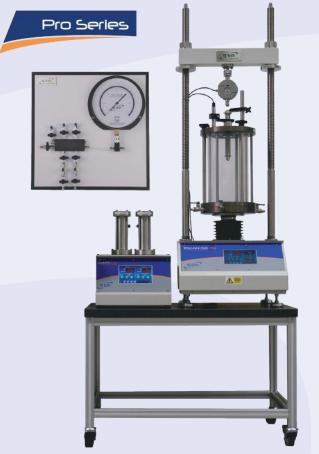
Pro Automatc Triaxial Testing System
